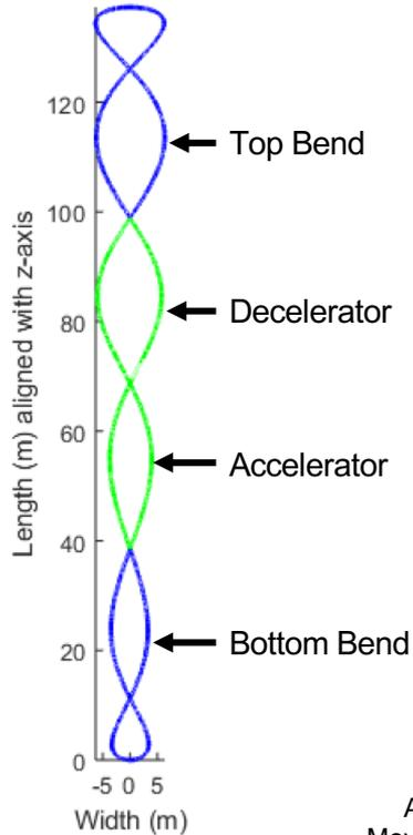
(a) Side View of Complete Beam Guide
