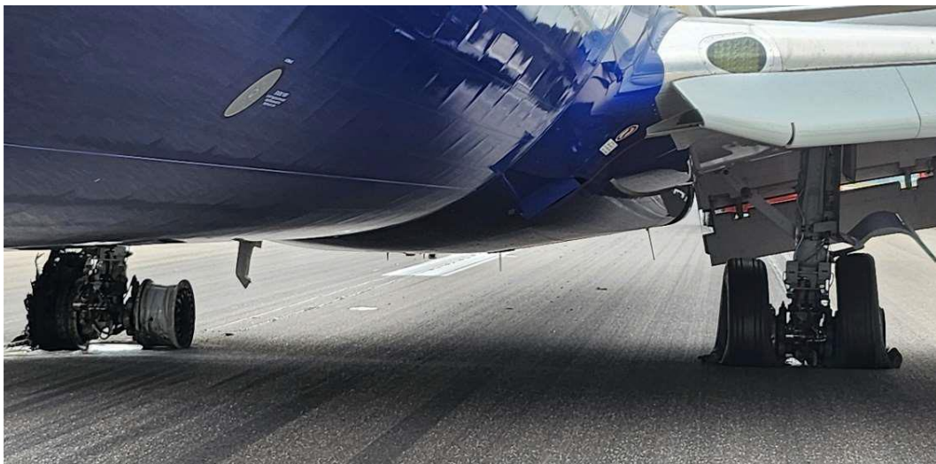
Photo 2 - Detail of wheel damage - front view (source: SACBO).
