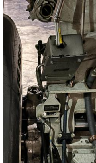
Photo 18 - air-ground sensor of the right MLG
