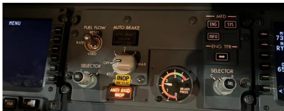
Photo 238 - Antiskid INOP warning light and the yellow label indicating the system is inoperative
