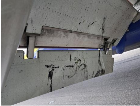
Photo 20 - Detail of damage to the right-hand 'inner flap'
