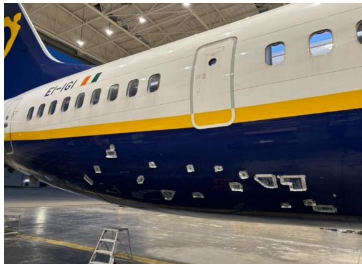
Photo 19 - Detail of damages to the right side of the fuselage
