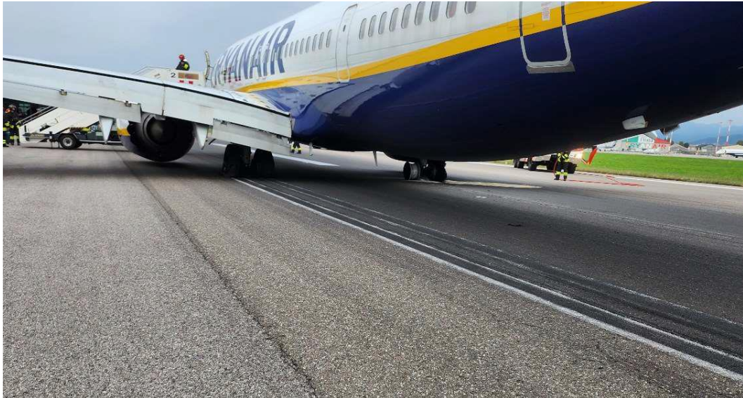
Photo 1 : close-up of wheel damage – rear view (source: SACBO).
