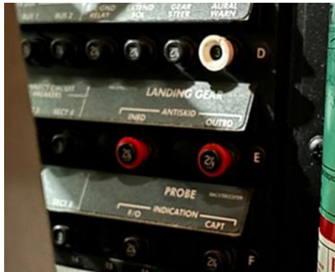
Photo 22 - detail of the removal and protection, using a 'collar', of the ANTISKID switches (INBOARD and OUTBOARD)
