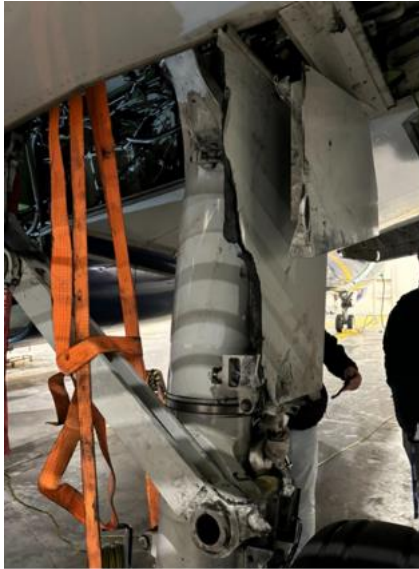
Photo 17: Structure, panels, linkages of the right MLG
