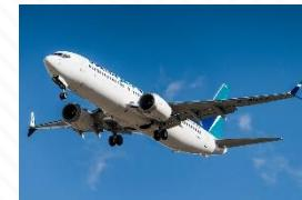
It is the last aircraft of the B-737 family presented by Boeing. The main change concerns the most powerful and efficient engines, as well as a modified avionics. The first flight for a B-737 MAX was made on January 29, 2016, 49 years after the inaugural flight of the B-737/100 of 1967.
