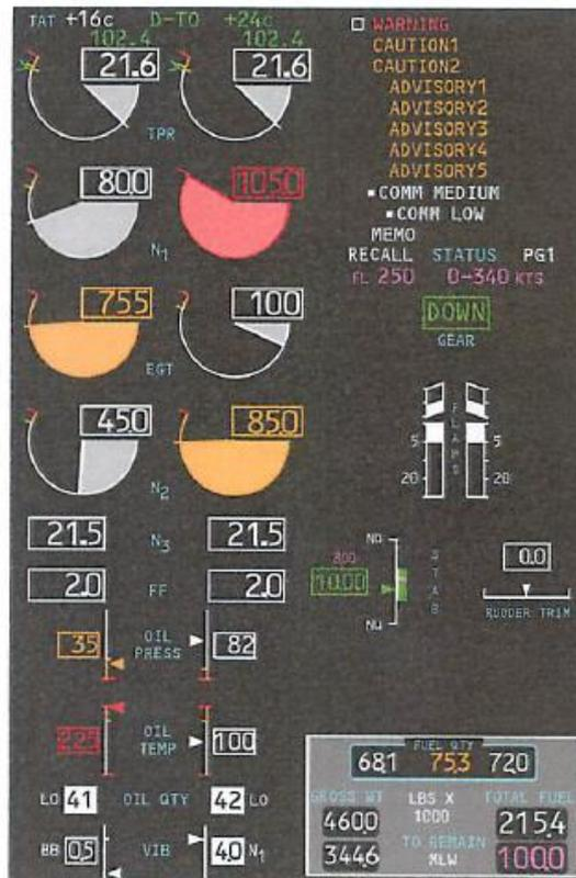
Figure 6: EICAS non-normal display mode.
