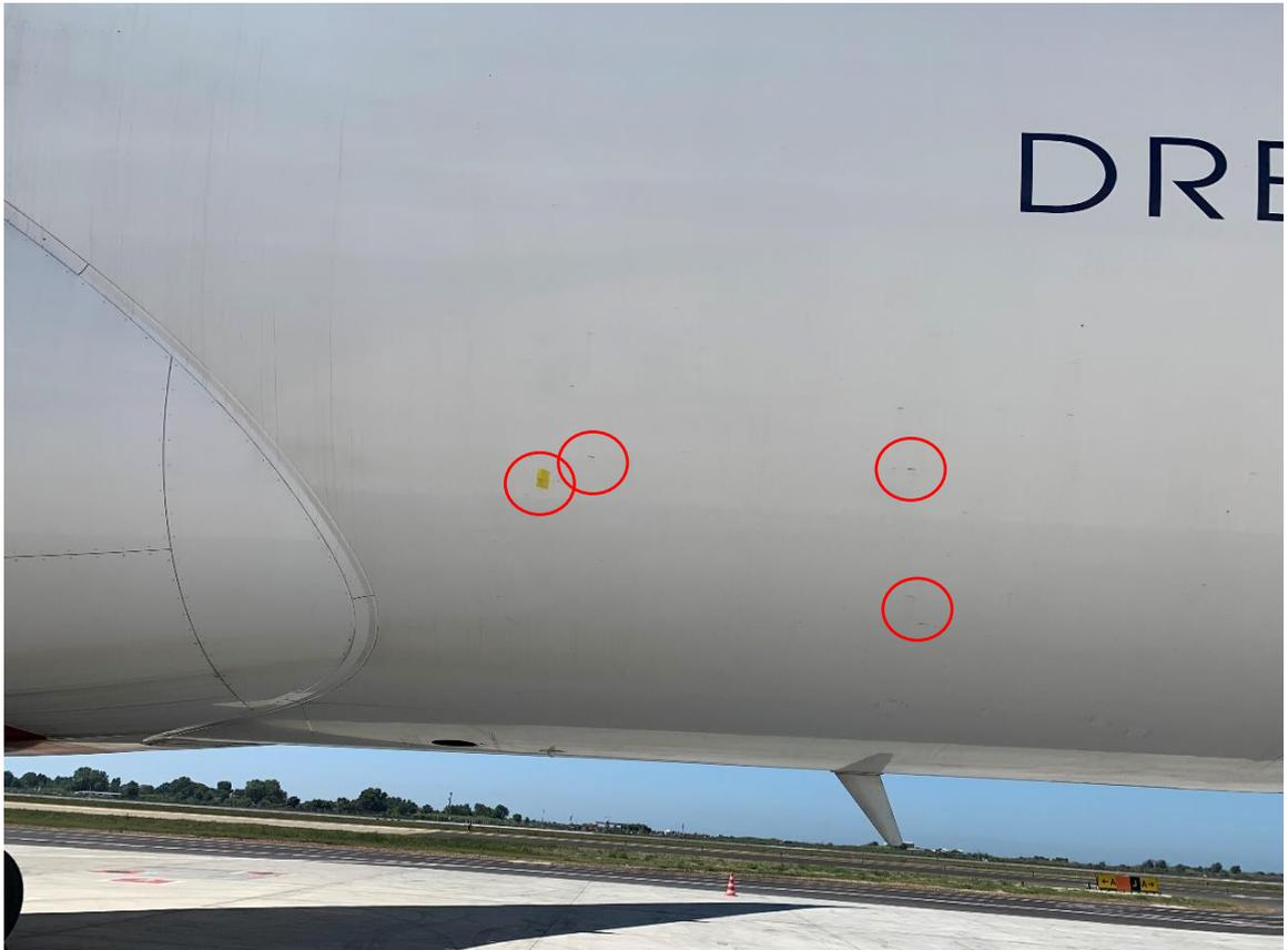
Photo 8: fuselage damage points.
