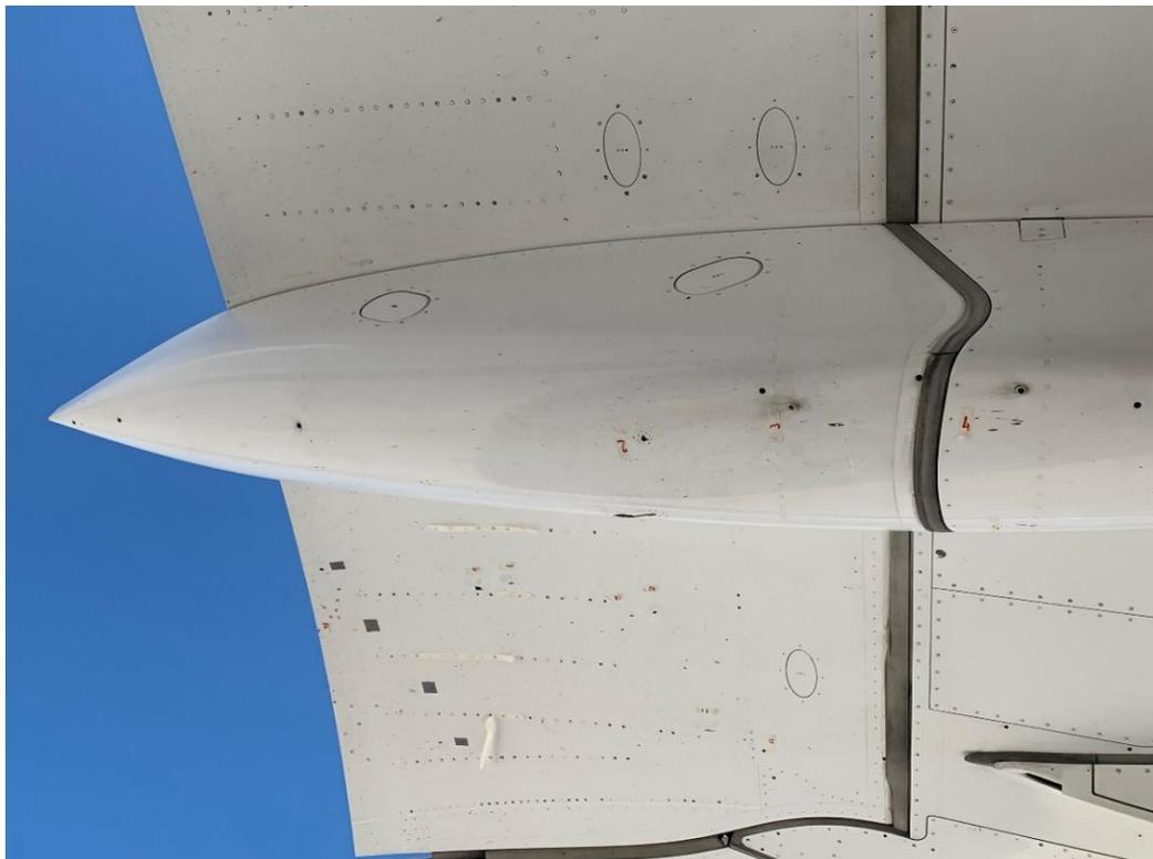
Photo 3: damage to the flap.
