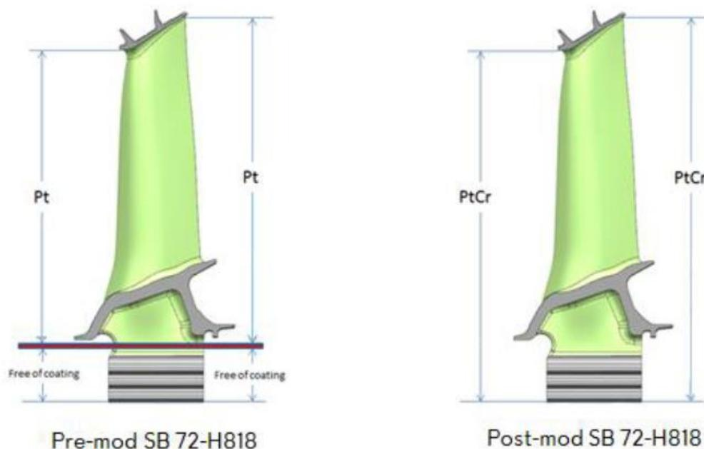
Figure 12: different configurations of the TRENT 1000 IPT blades (source Rolls-Royce).
