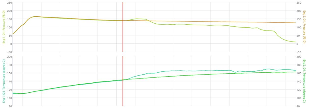
Figure 17: EAFR parameter selection, red line at the time 14.46'05'', comparison between ENG1 (left engine) and ENG2 (right engine).
