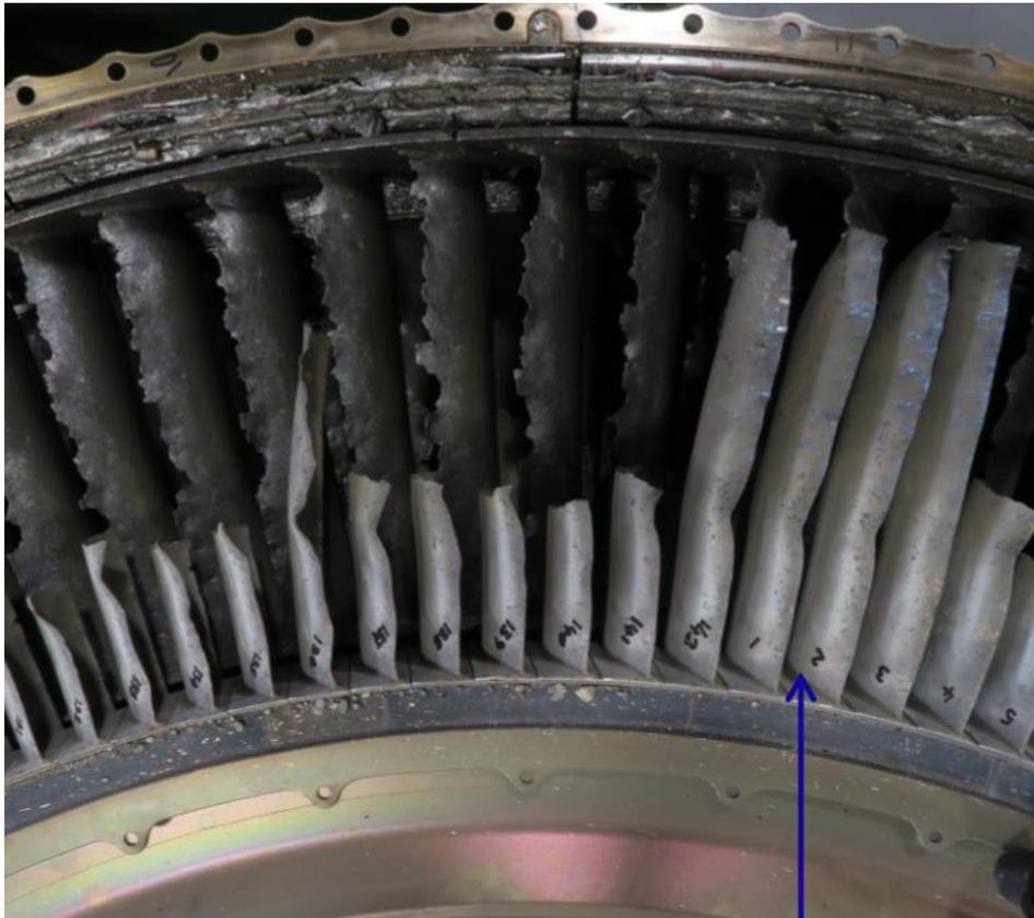
Photo 31: damage to the 6<sup>th</sup> stage LPT.
