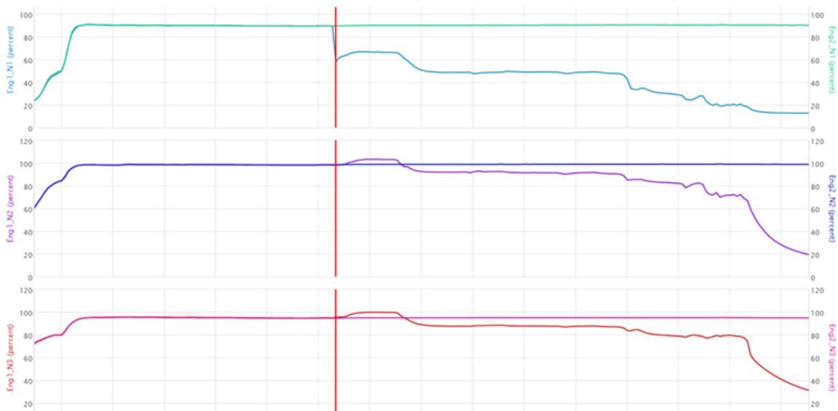
Figure 16: EAFR parameter selection, red line at the time 14.46'05'', comparison between ENG1 (left engine) and ENG2 (right engine).
