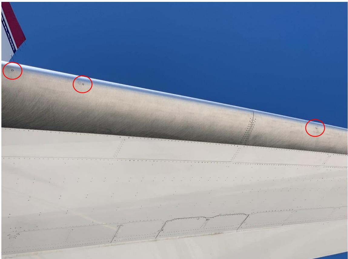
Photo 7: external damage of the horizontal stabilizer.
