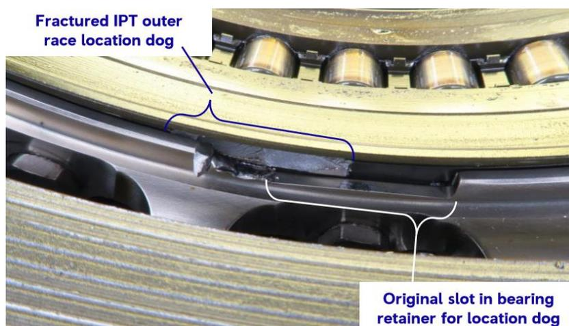
Photo 20: damaged anti-rotation slots.
