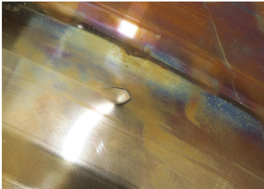
Photo 32: through thickness indentation 2<sup>nd</sup> stage LPT.
