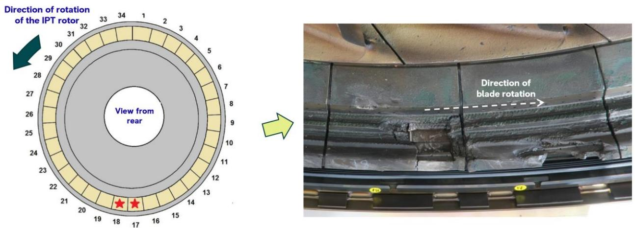
Figure 30: damage to the seal segment of the IPT stage.
