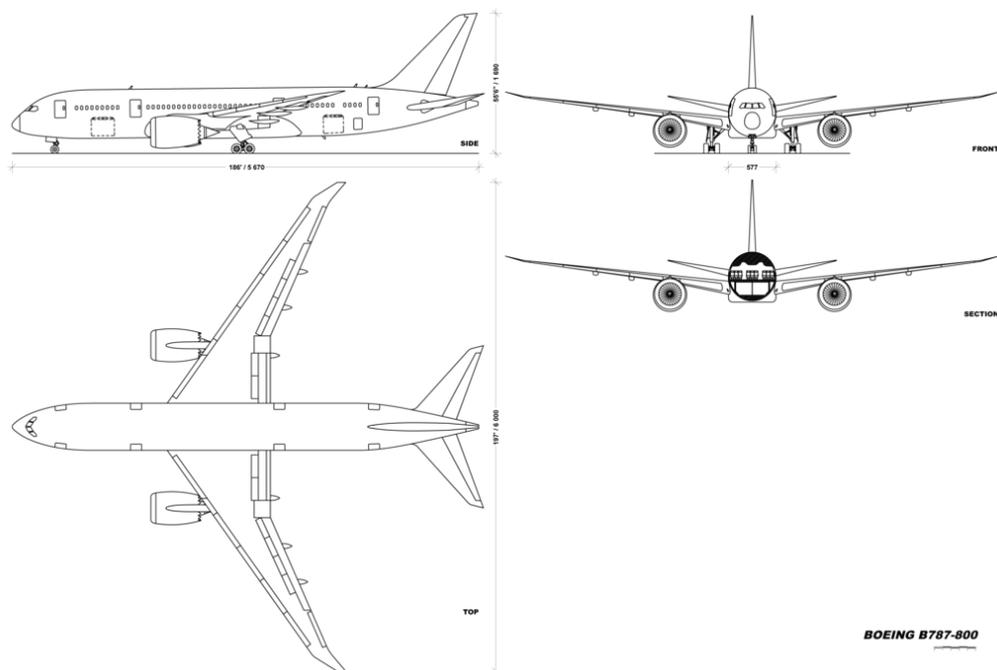
Figure 3: Boeing 787-8 schematic views.
