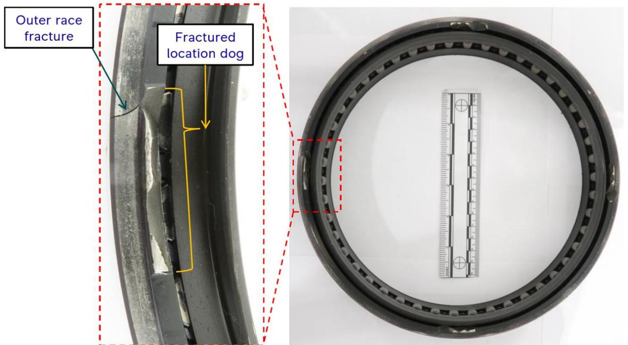
Photo 18: damaged (anti-rotation) location dogs.
