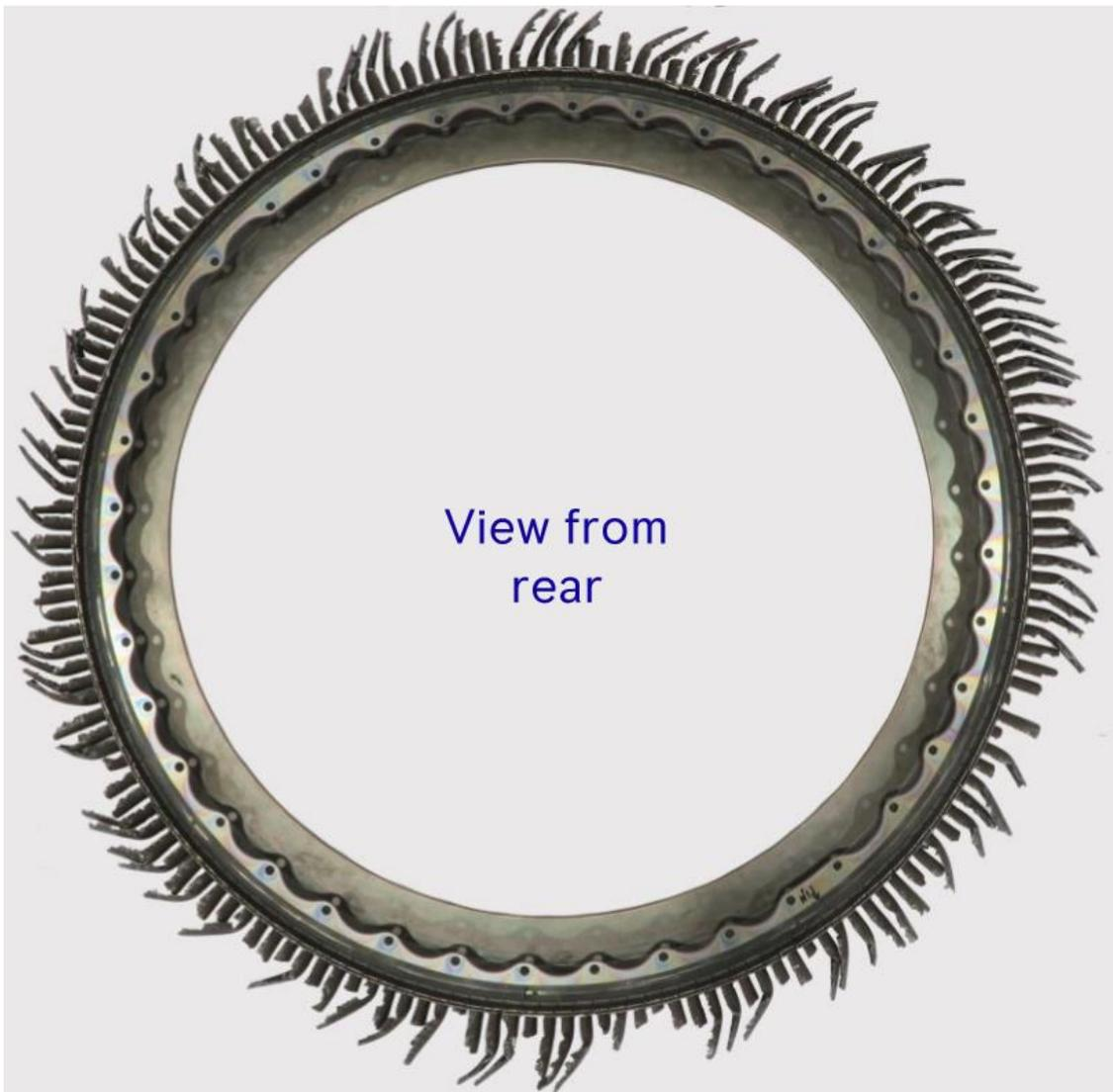
Photo 24: 1st stage LPT rotor damage.
