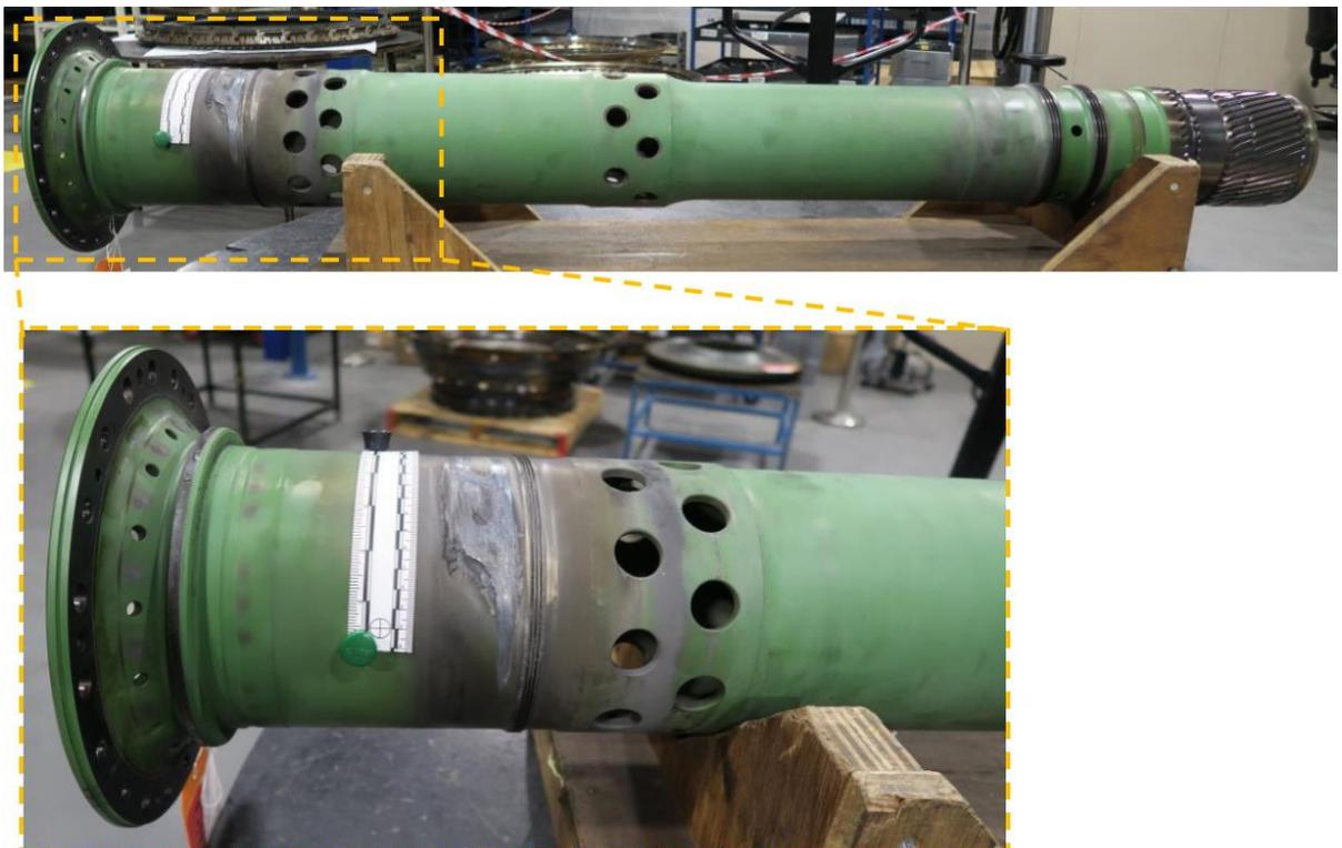
Photo 21: IPT shaft damage.
