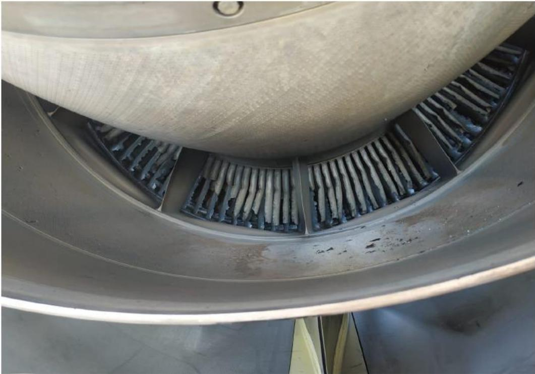
Photo 2: left engine damage as visible from the outside.
