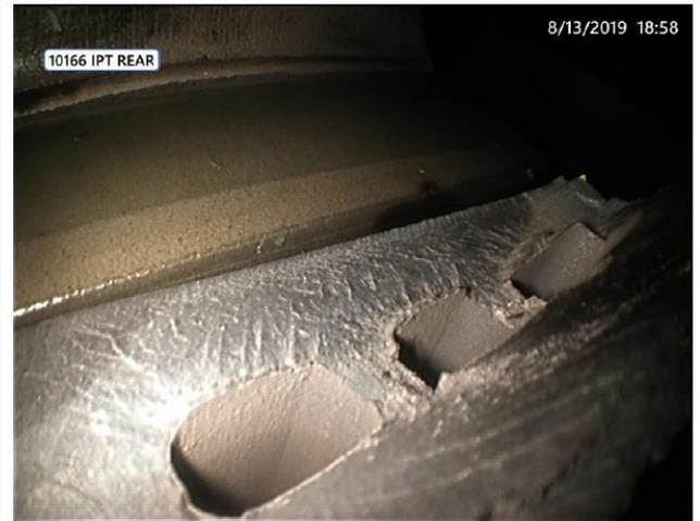
Photo 10: fracture surface of the primary damage consisting of the detachment of an IPT blade which led to the breakage of the adjacent one and then the further damage to the engine as described in paragraph 1.16.
