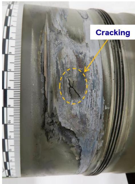
Photo 22: IPT shaft damage.
