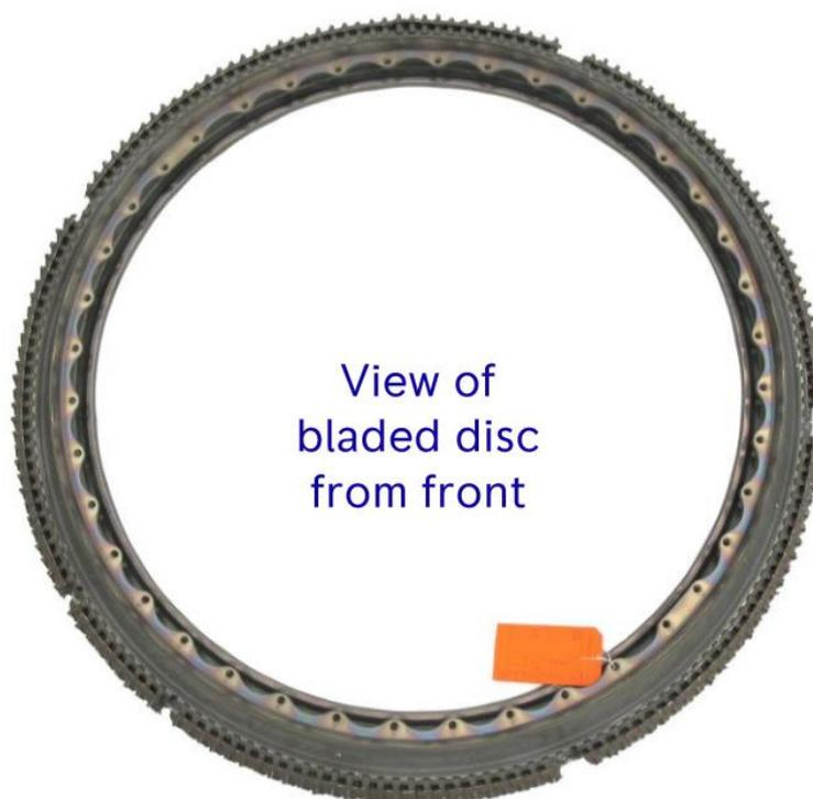
Photo 26: 2nd stage LPT rotor damage.
