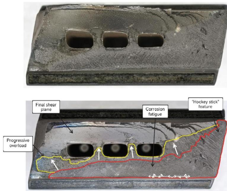
Photo 34: fracture surface.
