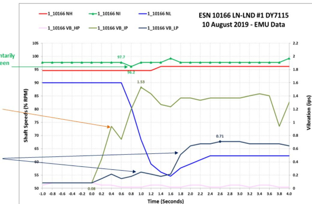
Figure 21: reconstruction of the sequence of events based on the EMU parameters (source Rolls-Royce).
