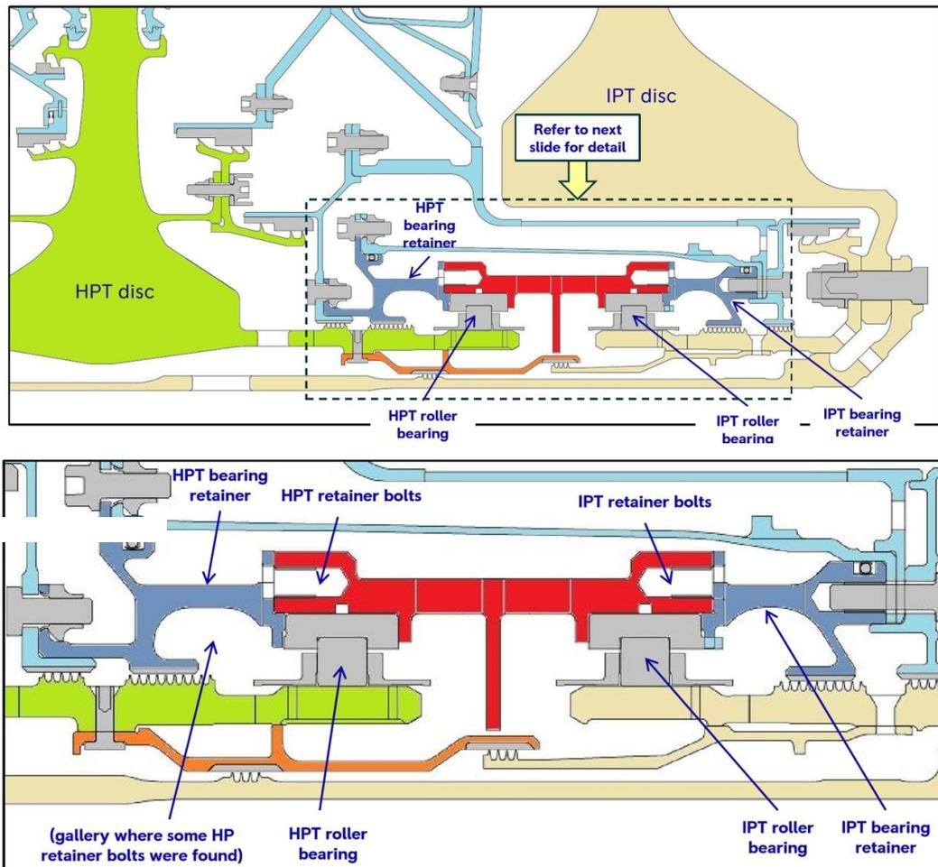
Figure 31: HP/IP bearing housing diagram.
