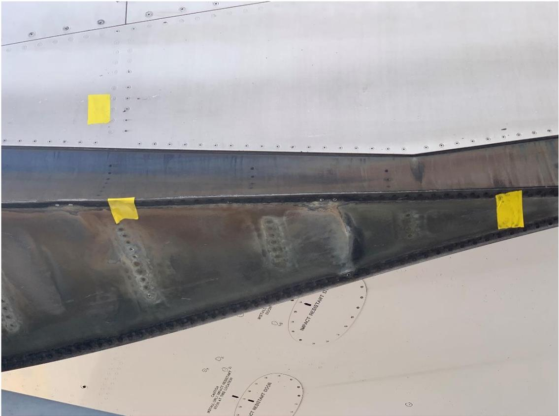
Photo 6: damage to the aft pylon fairing.
