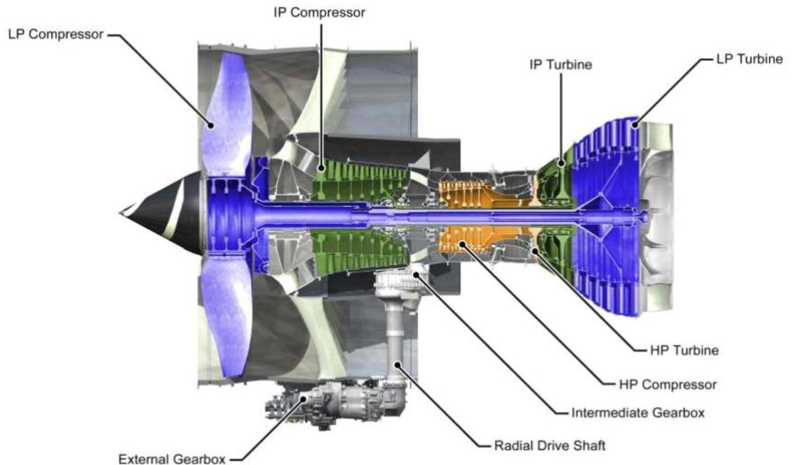
Figure 8: TRENT 1000, schematic view (source Rolls-Royce).
