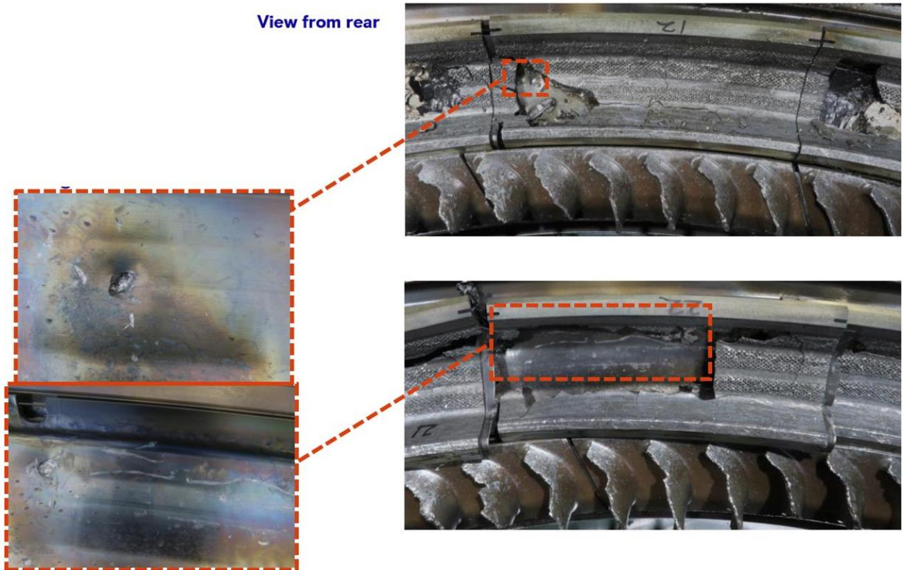
Photo 27: damage to 2<sup>nd</sup> stage LPT seal segments.
