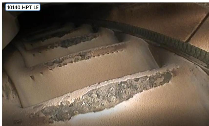
Photo 39: erosion on the HPT blades.
