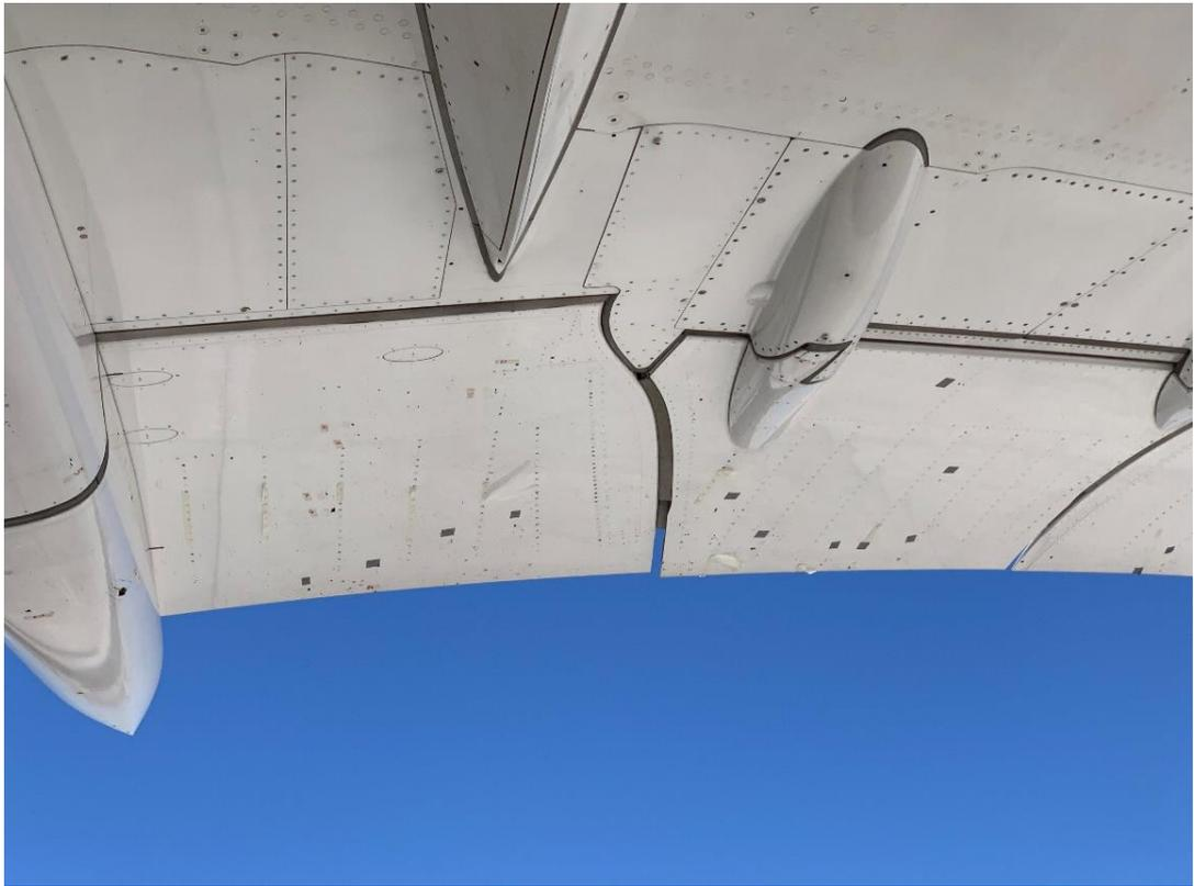
Photo 4: damage to the flap.
