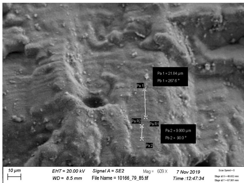
Photo 38: measurements for the calculation of striation spacing.
