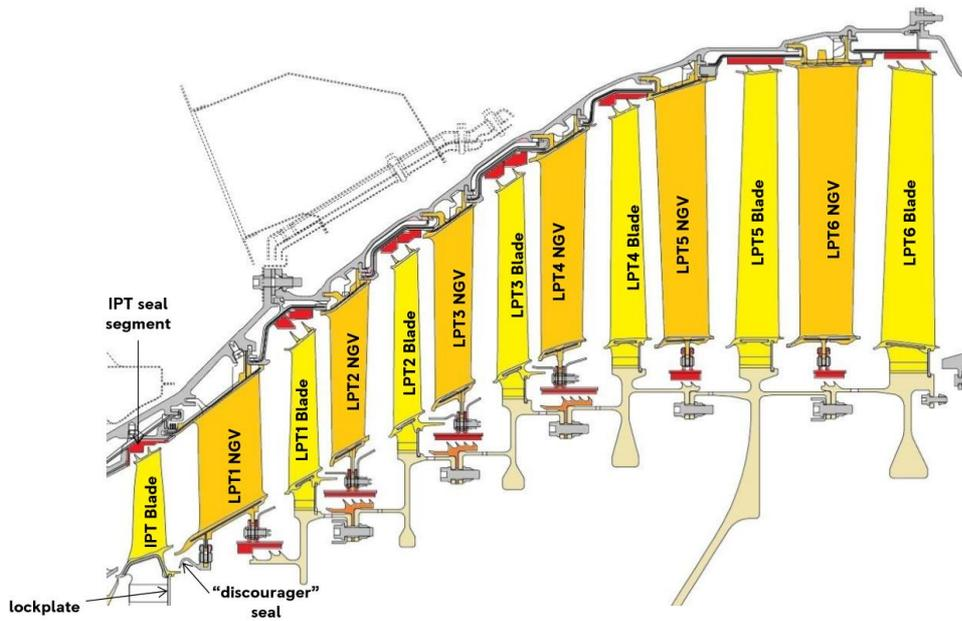
Figure 28: detailed diagram of IPT and LPT stages.
