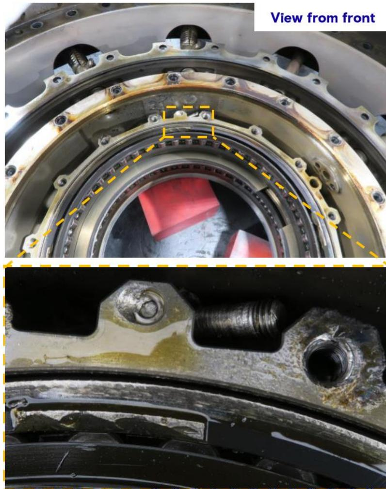
Photo 19: deformation of the holes for the HP bearing fixing bolts.
