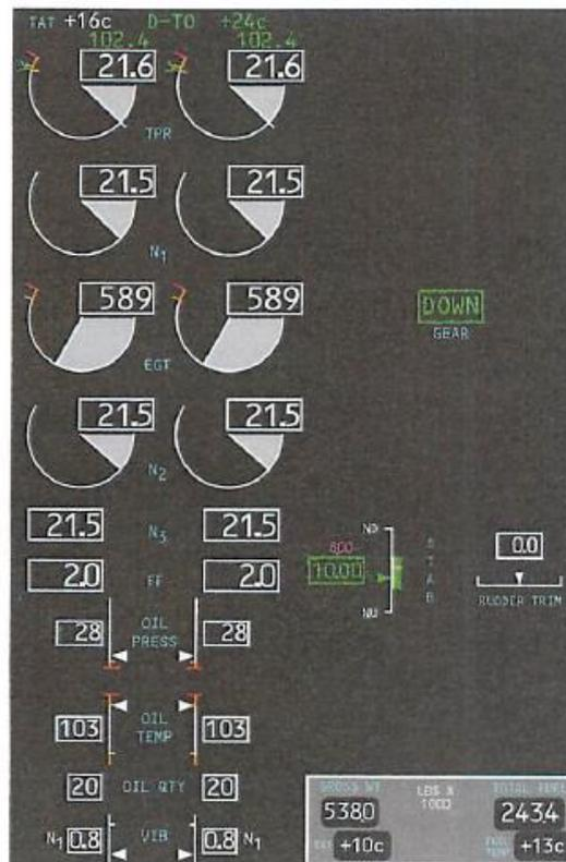
Figure 5: EICAS normal display mode.
