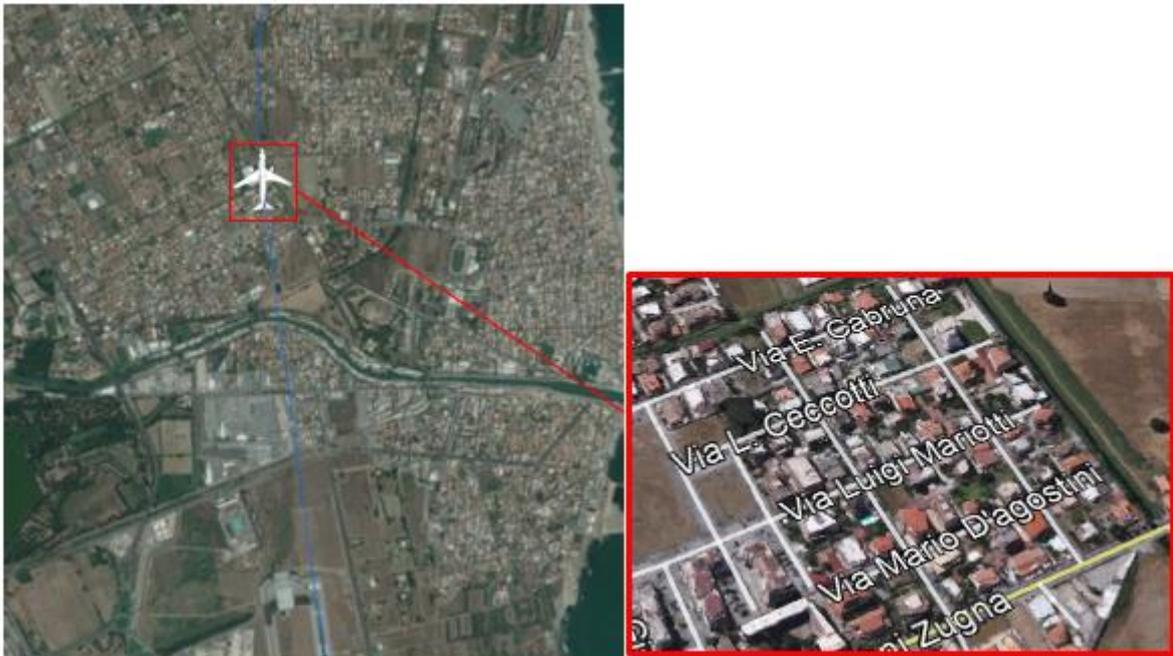
Figure 2: position of the aircraft at the time of activation of the discrete FDR parameter “Eng1 Vib Warn”; detail of the streets where most of the turbine blade fragments were found.
