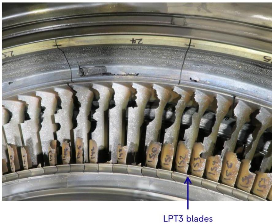
Photo 28: LPT 3<sup>rd</sup> stage damage.
